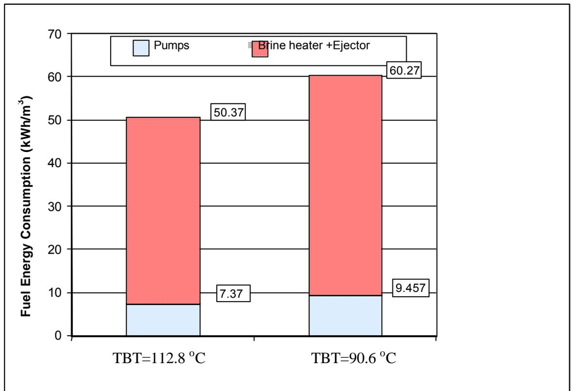
Figure 4. Fuel energy consumption of an MSF distiller coupled to a back-pressure power generation plant.
