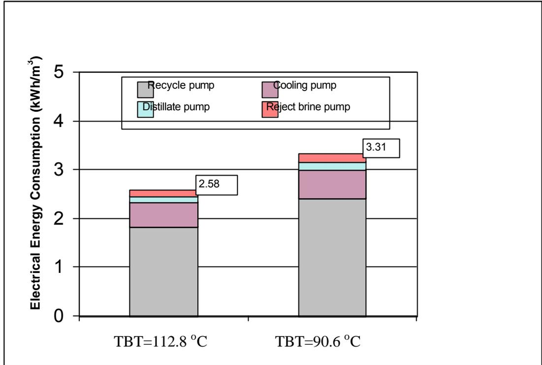
Figure 5. Breakdown of MSF electrical energy consumption.
