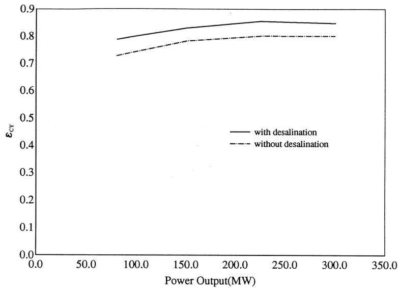
Fig. 7.  $\epsilon_{CY}$  vs. power output.
