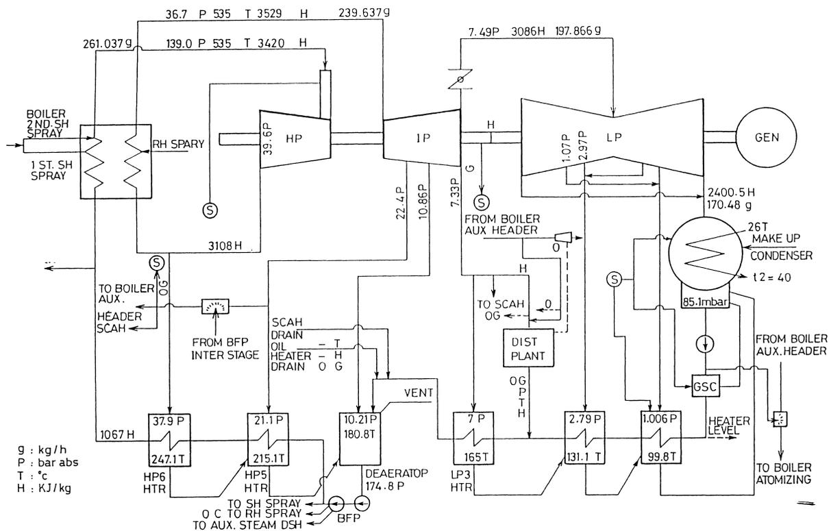
Fig. 2. Single purpose steam power plant.
