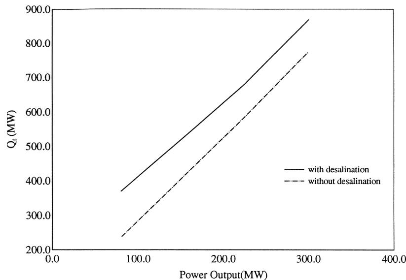
Fig. 4. Fuel energy vs. power output.
