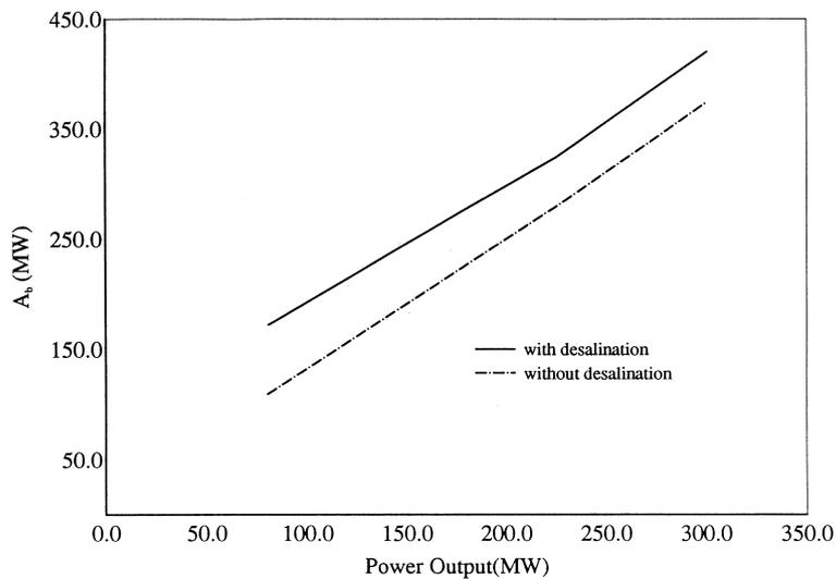
Fig. 6. Available energy given by the boiler vs. power output.
