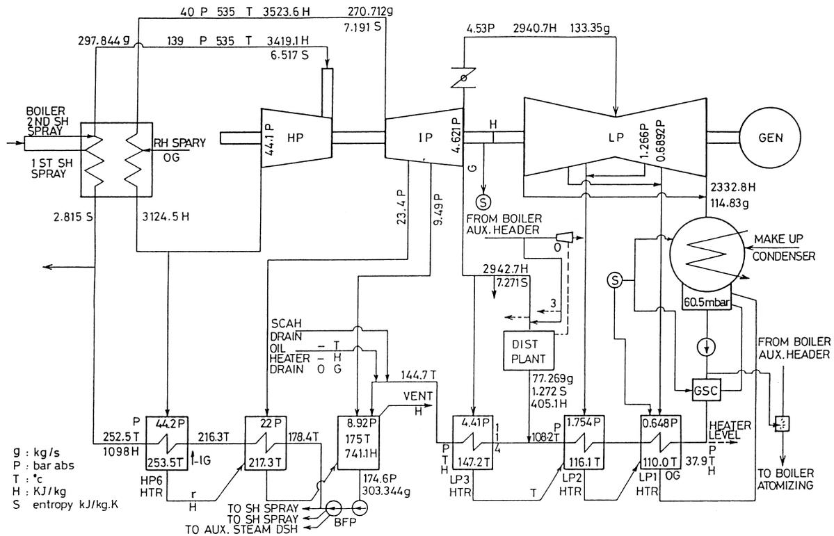
Fig. 3. Dual purpose (power-desalting) steam plant.
