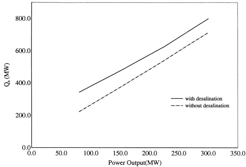
Fig. 5. Boiler heat output vs. power output.
