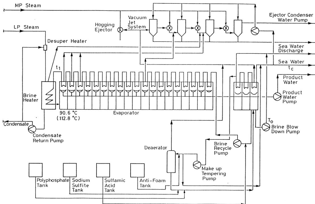
Fig. 1. Reference multi-stage flash desalination unit.
